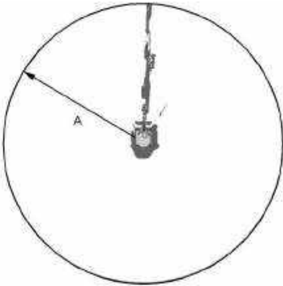
Illustration 52 g06321873 Top view of the machine, ground level visibility, with available left side mirror and right side mirror (A) 12 m (39 ft)
