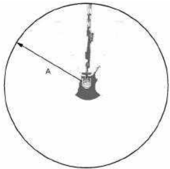
Illustration 53 g06321901 Top view of the machine, ground level visibility, with available left side mirror and right side mirror (A) 12 m (39 ft)
