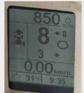
PUMA MULTICONTROLLER MODELS: THE RANGE AND GEAR SELECTIONS ARE CLEARLY SHOWN ON THE A-PILLAR DISPLAY
