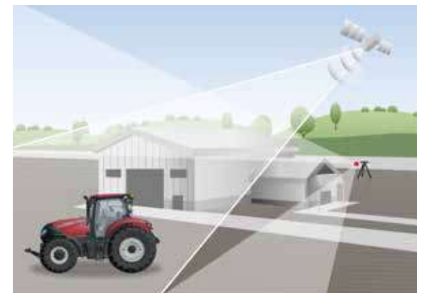
xFill bridges RTK+ signal losses of up to 20 minutes
